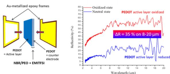
Fig. 1: (left) EED device assembled. (right) Mid-IR dynamic within the 2-20µm range
