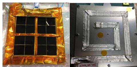
Fig. 2: Electroemissive Radiator front (left) and back (right)
